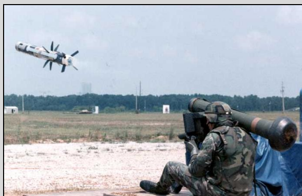
Figure 16.7: HEAT isn't just for chemists – it's also an acronym for High Explosive Anti Tank weapons. Shown here is the FGM-148 Javelin anti-tank missile being fired by a member of the American armed forces.
