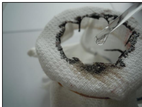
Figure 10.3: Sulfuric acid is so spectacularly corrosive that it can even burn through a thin cotton towel.
